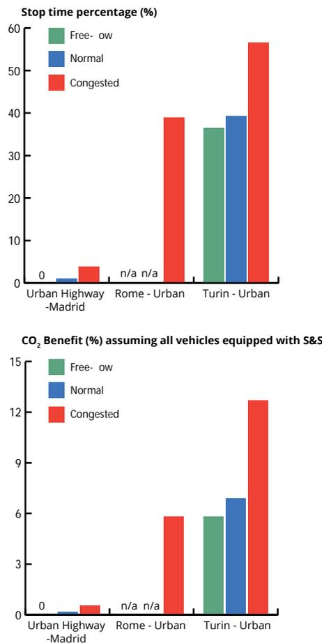
We also examined the combination of S&S together with UTC in two cities. This is a typical example that the combined benefit of two ICT measures is not their arithmetic sum. The following figure shows that UTC and S&S at congested conditions offer maximum benefits, which are though 10% lower of the arithmetic sum of the benefit of both measures. Still, this is a very substantial benefit.
