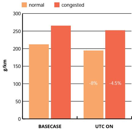
Impact of UTC on average CO<sub>2</sub> emission levels per unit of distance travelled. The values refer to the average vehicle (including passenger cars, light commercial vehicles, buses, and trucks).
