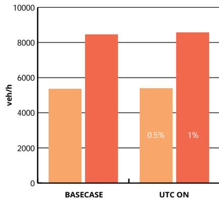
Slight increase in the traffic flow with the UTC system on.
