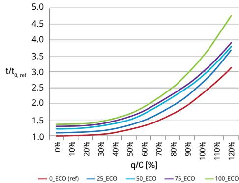
and Turin (urban network) by using the results of several micro traffic simulations with various degrees of eco-driving penetration. The following figure shows the new functions derived for urban driving and a summary of key macroscopic parameters is shown in the adjacent table.
