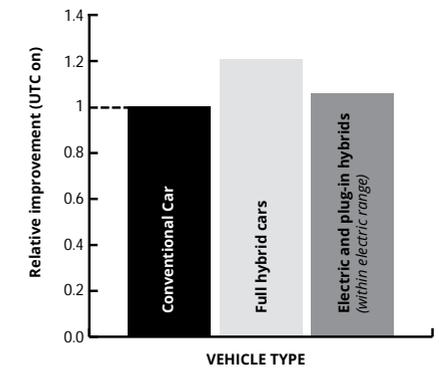
Relative improvement of CO<sub>2</sub> emissions with UTC system ON for different vehicle types, relative to conventional vehicles. The improvement for conventional cars has been assigned the value of one.
