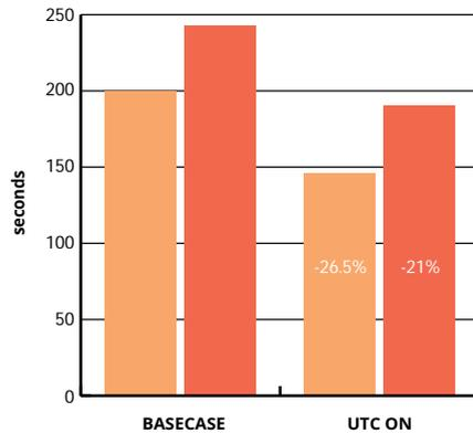
Drop in the travelling time [s] with the UTC system on.
