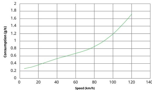
*Generalized fuel consumption function of speed used in the green navigation routing optimization problem for passenger cars*
