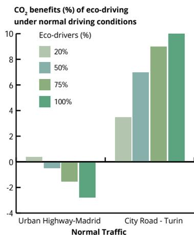
Small or even negative benefits of eco-driving may be likely in congested conditions: eco-driving may lead to an early saturation of the road, as the fraction of eco-drivers increases. This is shown in the following figure.
