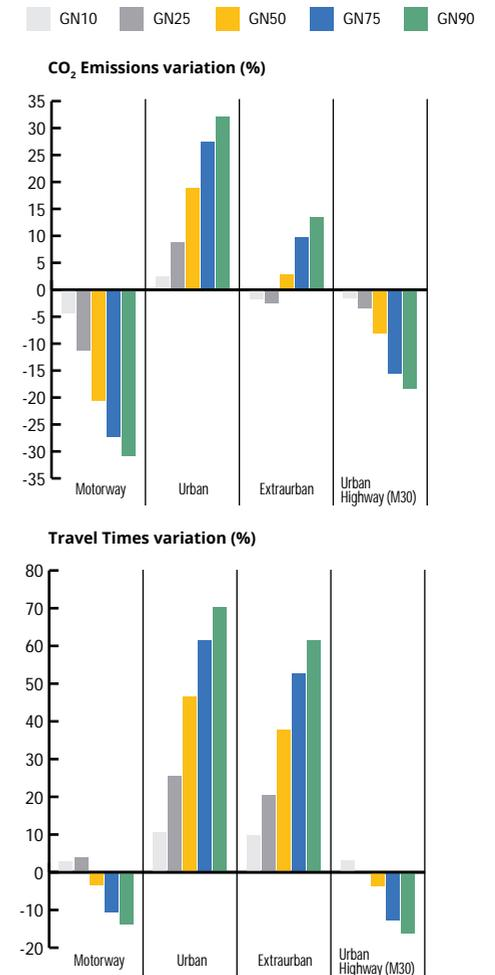
Example of variation of CO<sub>2</sub> emissions, traffic volume and travel time per road type in the case of congested traffic network in Madrid. To reduce fuel consumption routing shifts traffic from highways to secondary roads which results to significant increase of travelling time.
